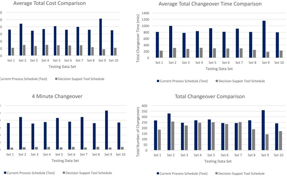
The logic implemented in our decision support tool helps to significantly reduce the total changeover time and cost resulting from a production schedule.
