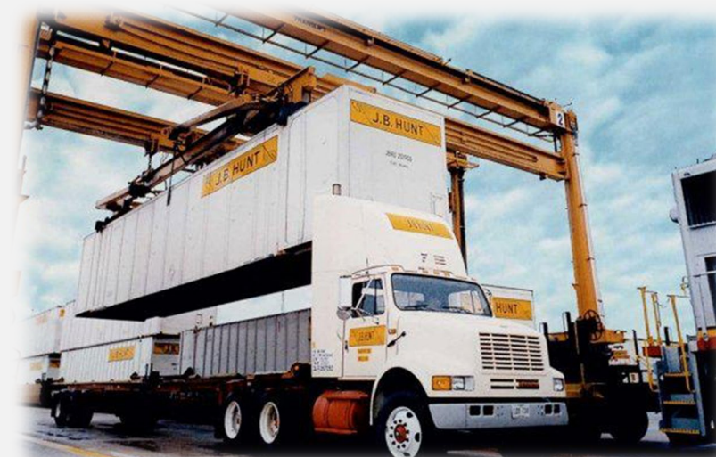
Container at a ramp being taken off of a truck chassis for placement onto a rail
