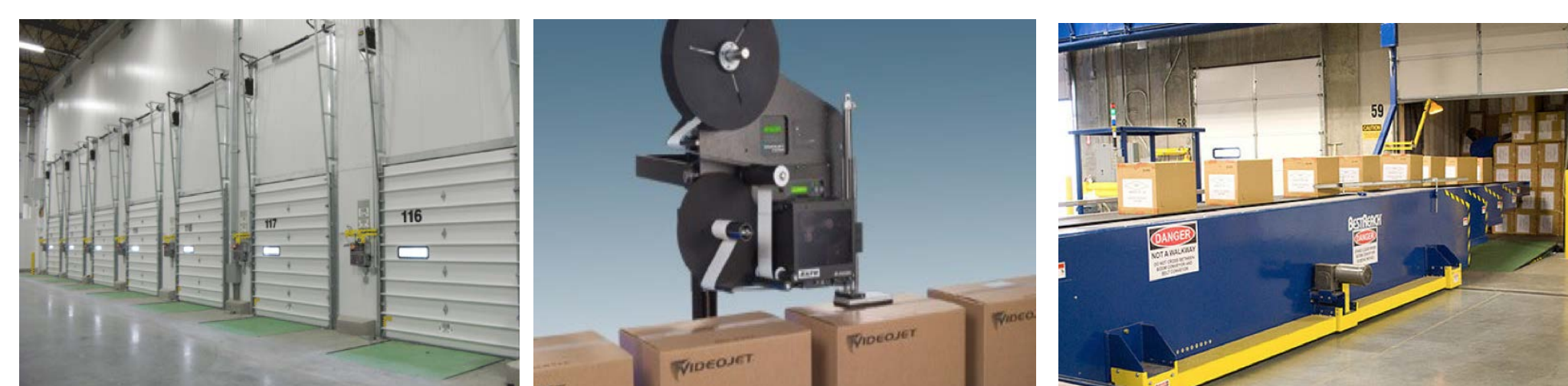
Figure 3. (left to right) A Normal Dock Door, an ACL, and an Extendable Conveyor
