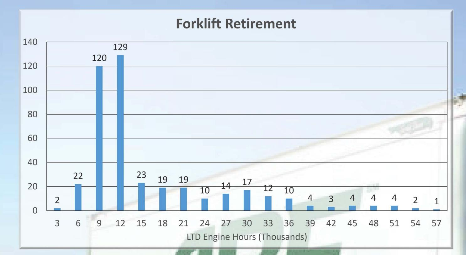
The group required data on when forklifts were being retired. A macro in excel was created to calculate the retirement of forklifts by identifying the last station number a forklift had maintenance performed at. The macro then calculated the life – to – date (LTD) engine hours and service years upon retirement. The histogram displays the LTD engine hours accrued upon retirement and the count of forklifts for each interval.
