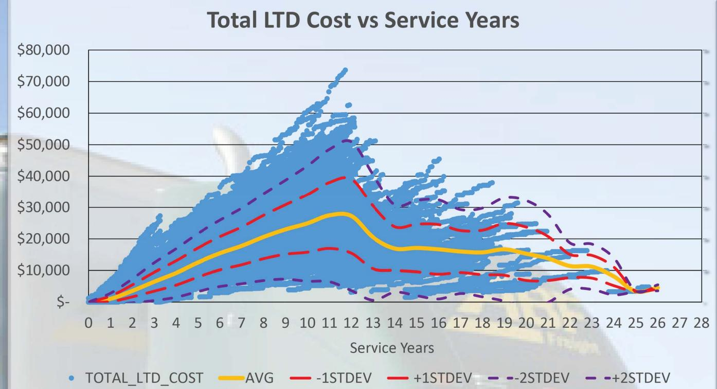
In order to calculate the optimal replacement interval for ABF Freight's forklifts, the operation and maintenance cost (O&MC) for each year of service had to be calculated. As the graph shows, there is a wide variability in the O&MC. To account for this variability, a range of two standard deviations must be made. Multiple optimal replacement intervals will be calculated using the range of O&MC.
